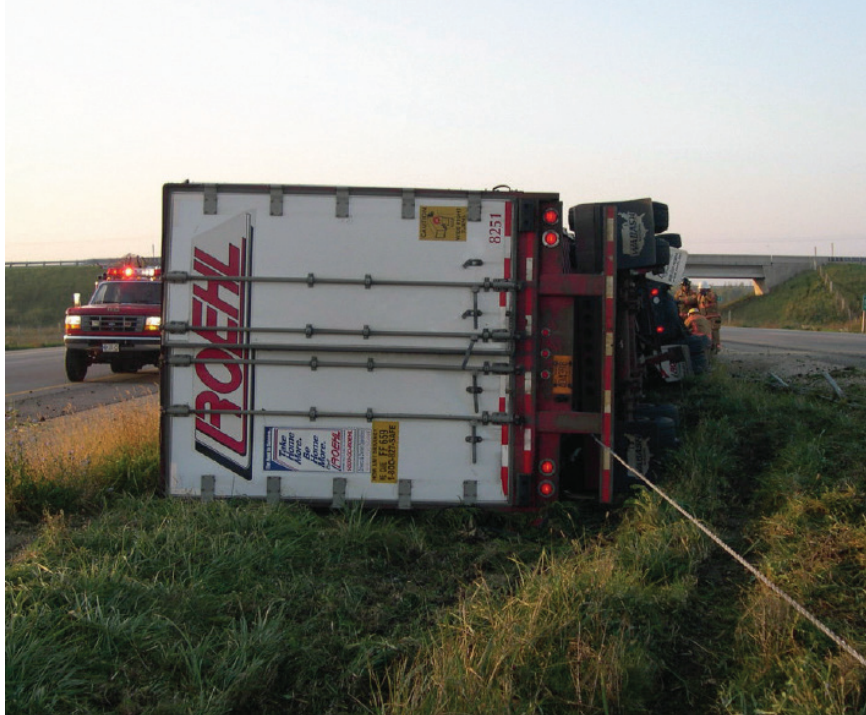
Figure 7. Mr. Krull's Tractor-Trailer Captured by a Cable Median Barrier on Hwy 41 in Wisconsin
